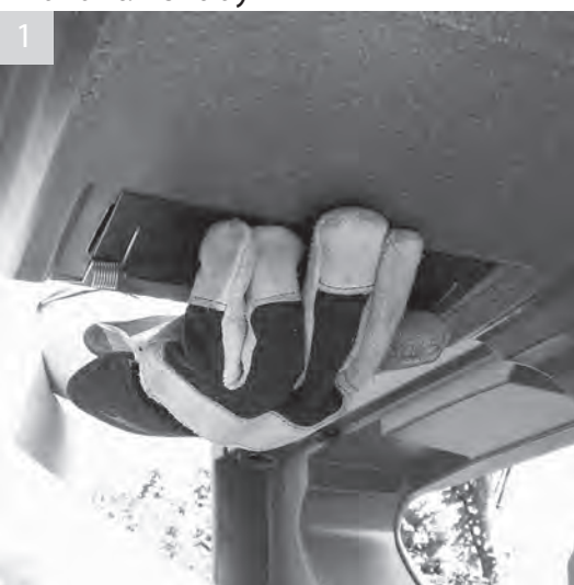
1 From door aperture reach inside the bin and grip the lip on the ashtray hinge flap
