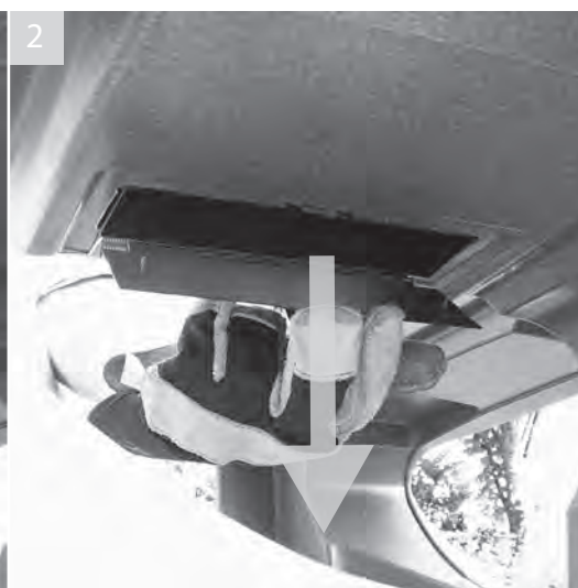
2 Pivot the ashtray flap downwards until it is vertical. Contents will fall into the liner below
