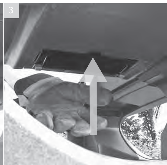
3 Once the contents of the ashtray has fallen into the liner release grip, the sprung hinge will return the flap to its closed position
